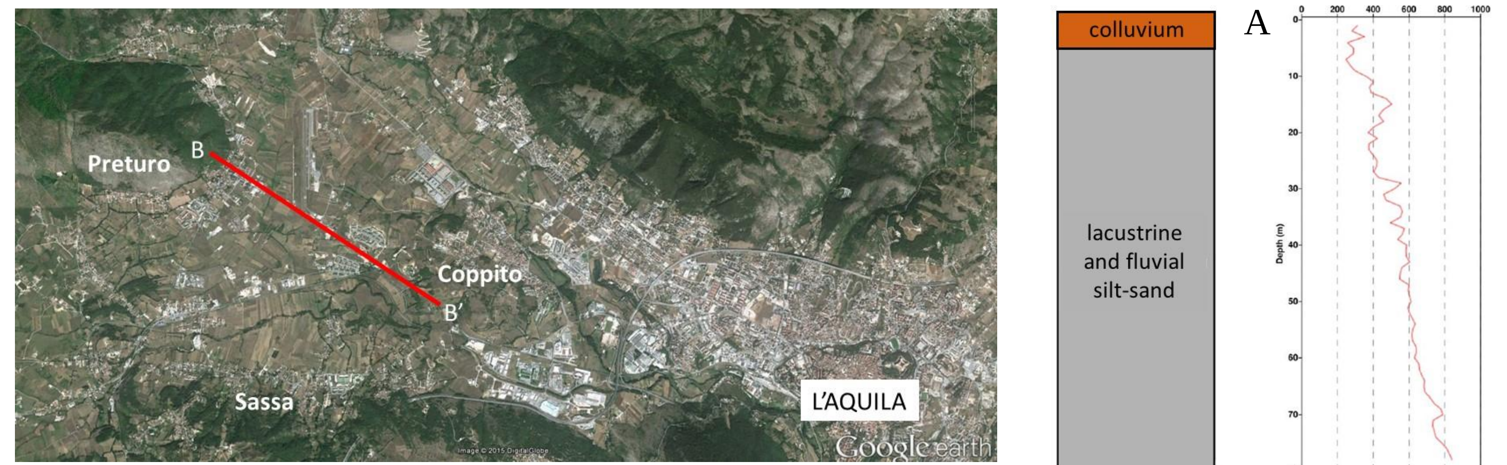
Fig. 1 – Location of the studied area. The red line refers to the Preturo-Coppito geological section representative of the subsoil model of Western L'Aquila Plain and which was used for the 1D and 2D numerical modeling (see Fig. 2).
