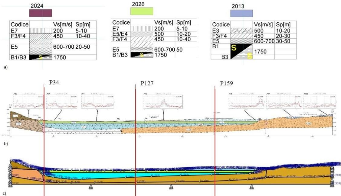
**Fig. 2** - a) MOPS stratigraphies used in 1D and 2D modeling. B1 - structurally ordered layered rocks; B3 - layered rocks characterised by strong competence contrast due to alternating layers of rocks and pelites; E3 - sandy gravel; E5 - gravelly sand-; E7 - sandy silt-; F3 - clayey silt -; F4 - silty clay (AA.VV., 2014); b) section B-B' (Preturo-Coppito): AA.VV., 2014; c) section B-B': mesh obtained with the software LSR 2D.
