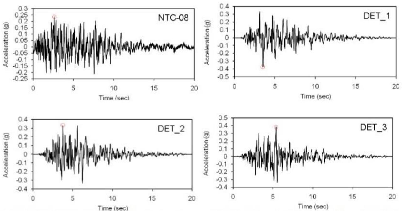
**Fig. 1** - DET\_1, DET\_2, DET\_3 and NTC: the four different input accelerograms used in the 1D and 2D numerical modeling (Gruppo di Lavoro MS-AQ, 2010).
